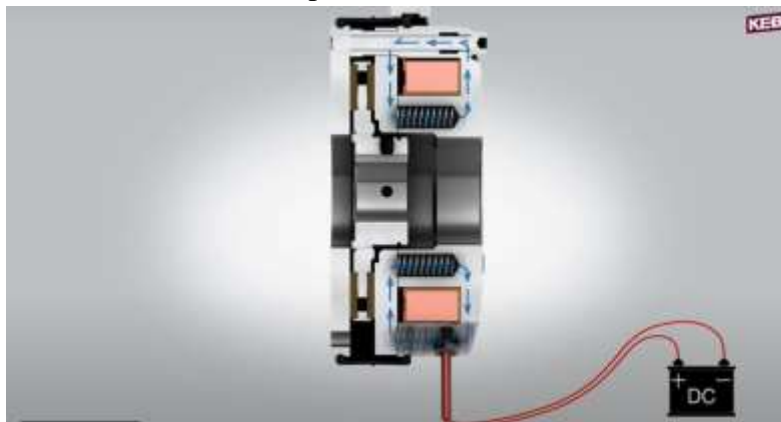
Figure 13 - Failsafe involving an electromechanically mechanism
